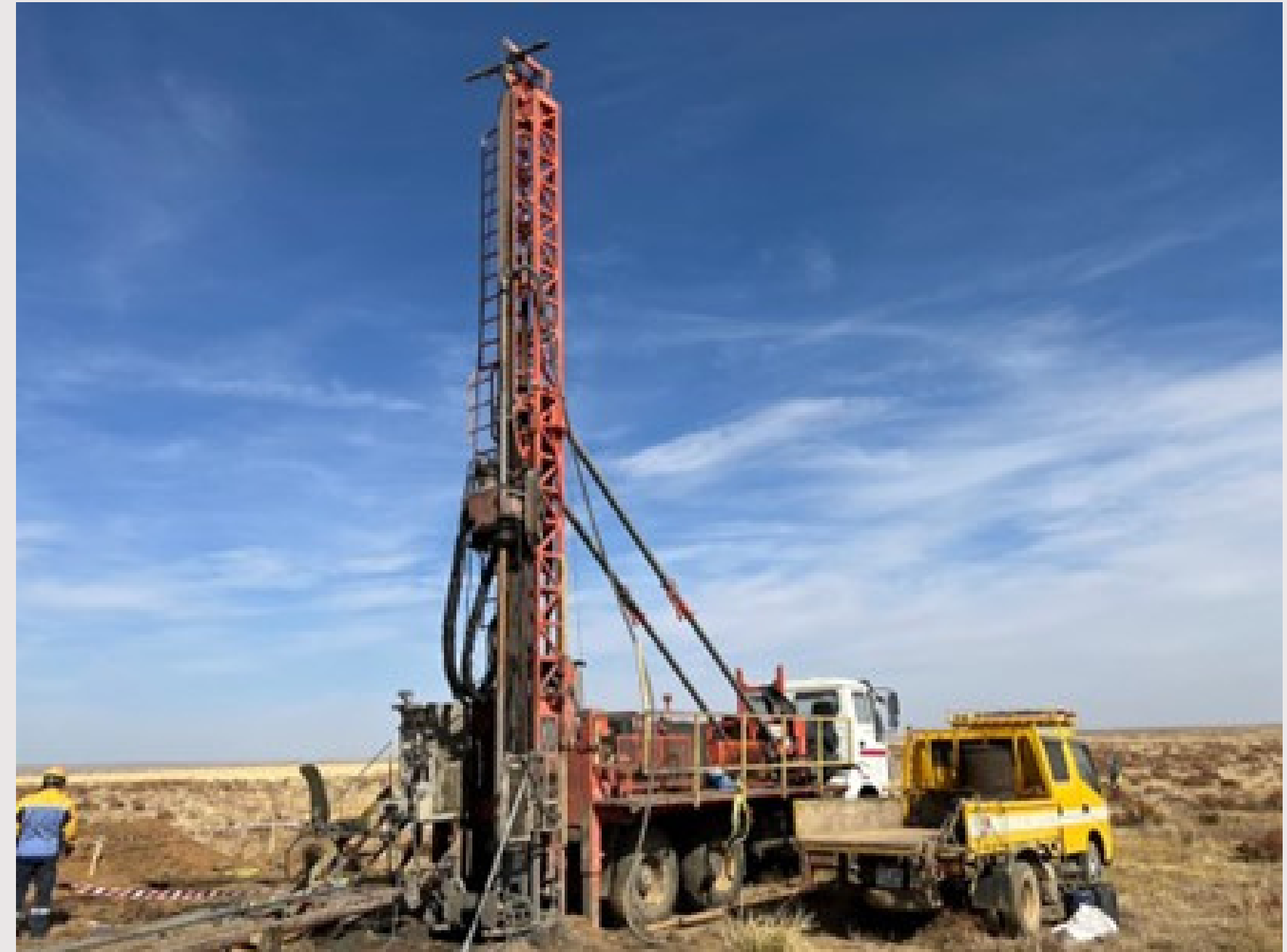
Diamond core drilling at UNDH-02
